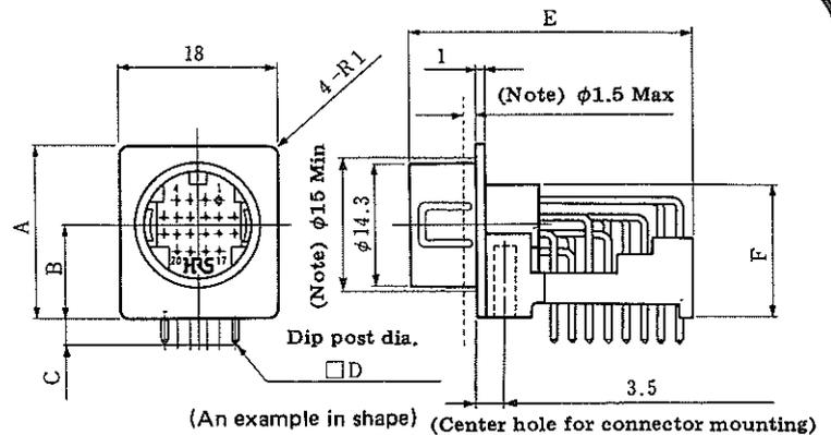
Note: Set up the mounting panel thickness less than 1.5mm, mounting whole more than  $\phi 15$ mm.
