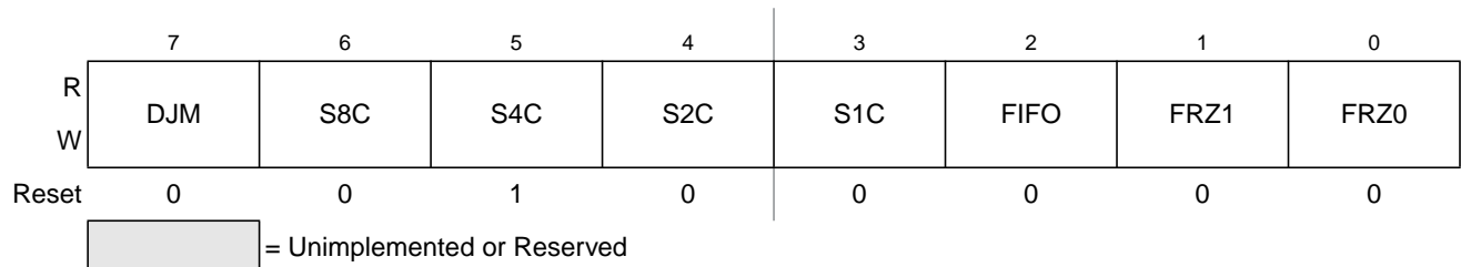
Figure 10-7. ATD Control Register 3 (ATDCTL3)
