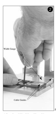
Adjust the width of the cable guides on the 10980-3 locator plate to correspond to the connector. Use width gauge 10983-XX for connectors having XX positions. Remove the width gauge when finished.
