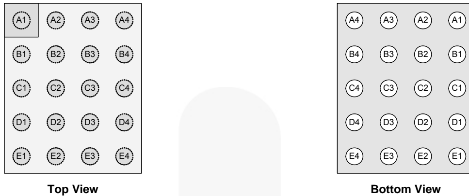
Figure 4. WLCSP-20 Pin Assignments
