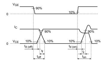
Note 2: Switching loss measurement waveforms
