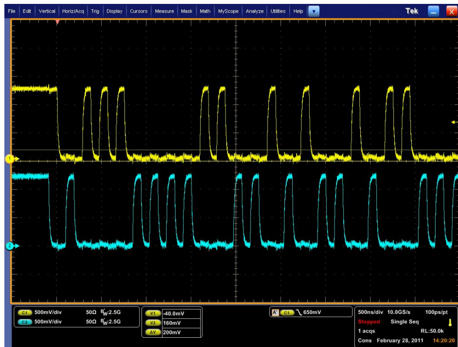
Figure 5. EMI4172 MIPI D-PHY LP Mode Measured Results
