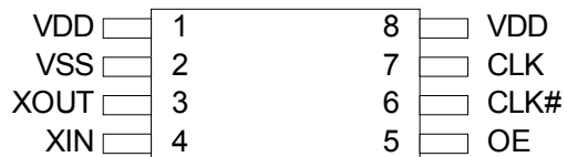
Figure 1. 8-pin TSSOP pinout
