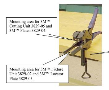
Mount the 3M<sup>TM</sup> Hand Press to a bench using the 3M<sup>TM</sup> Bench Clamp.
