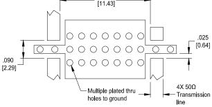
Dimensions are in Inches [Millimeters] X3DC08E2S Mounting Footprint
