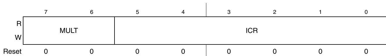
Figure 11-4. IIC Frequency Divider Register (IICF)
