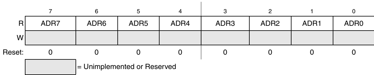
Figure 9-7. Data Result Low Register (ADCRL)
