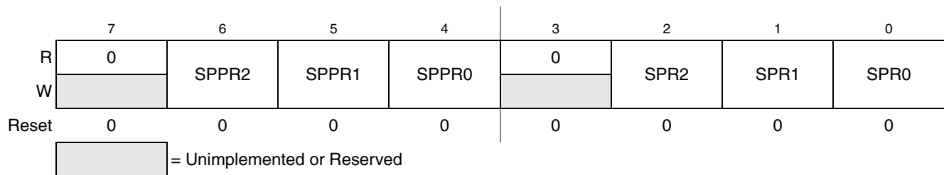
Figure 15-7. SPI Baud Rate Register (SPIBR)
