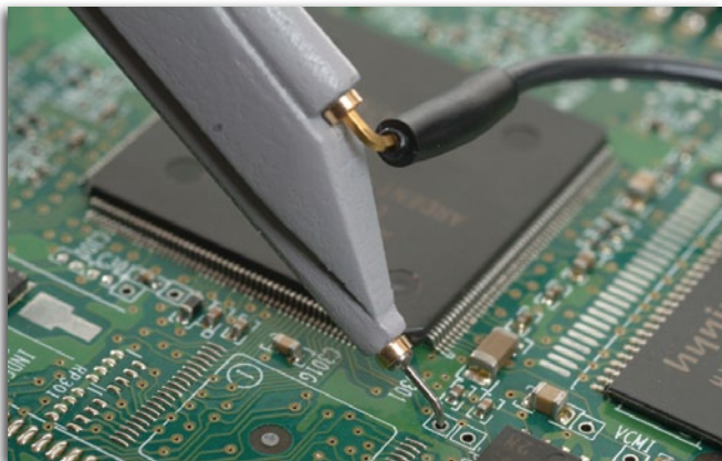
Hard-to-reach spaces can be be probed with the Bent Sharp Tip and can be used with a range of ground leads like the flexible Short Right-Angle Lead shown here.
