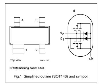
transistor consists of an amplifier MOS-FET with source and substrate interconnected and an internal bias circuit to ensure good cross-modulation performance during AGC.
