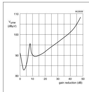
$V_{DS} = 5 \text{ V}; \ V_{GG} = 5 \text{ V}; \ f_w = 50 \text{ MHz}.$   $f_{unw} = 60 \text{ MHz}; \ T_{amb} = 25 \text{ °C}; \ R_{G1} = 120 \text{ k}\Omega.$
