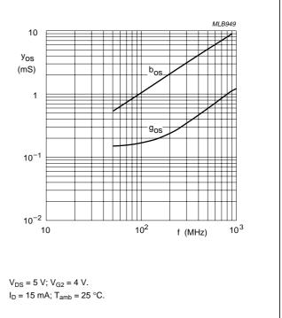
Fig.17 Output admittance as a function of frequency; typical values.
