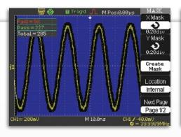
With built-in Pass/Fail Mask testing
