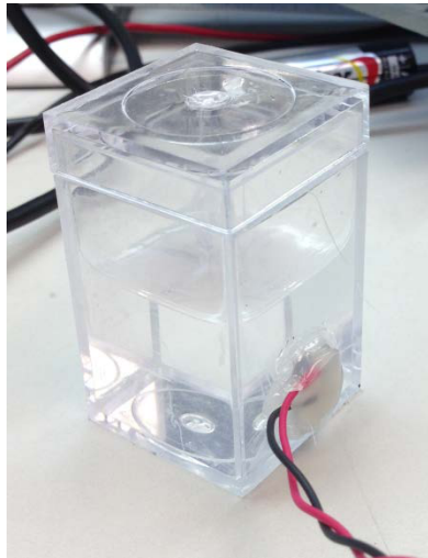
Figure 2. Water Container with 1-MHz Transducer
