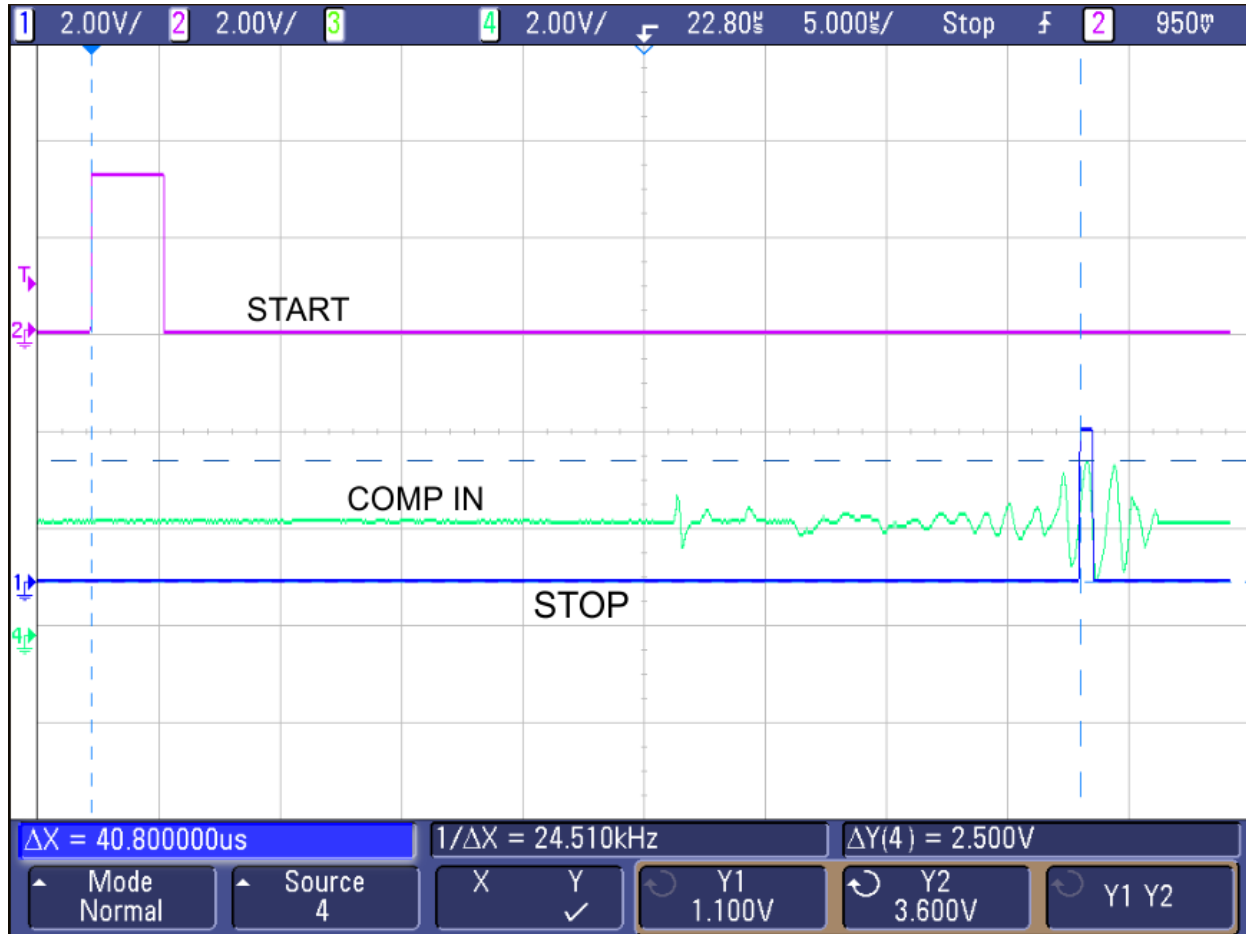
Figure 10. START, COMPIN and STOP Signals on Oscilloscope
