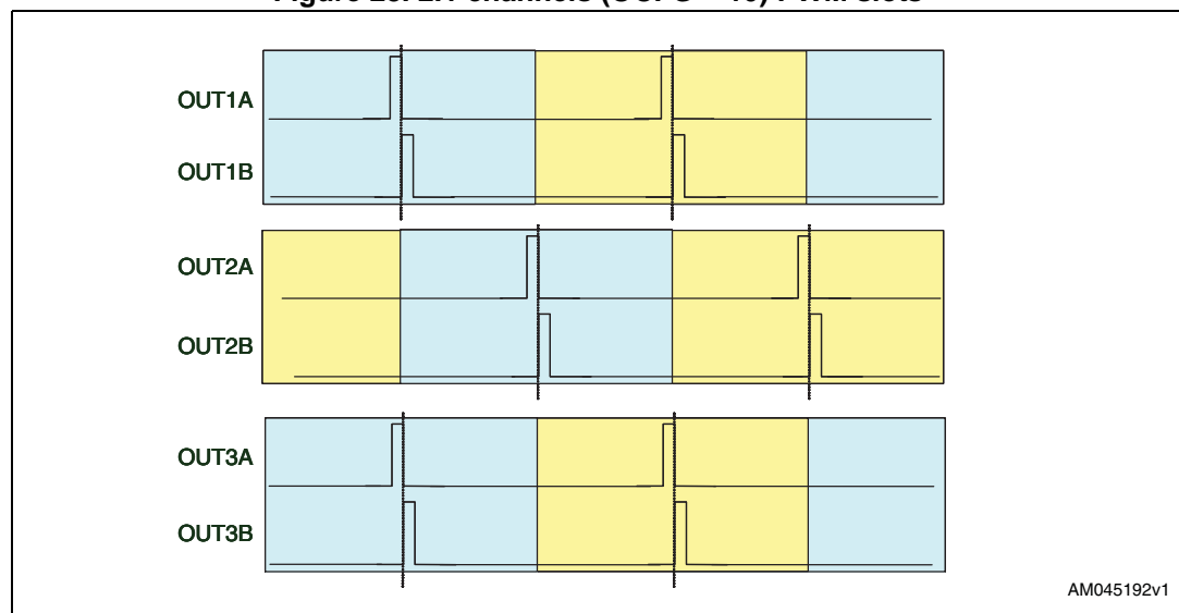
Figure 28. 2.1 channels (OCFG = 10) PWM slots
