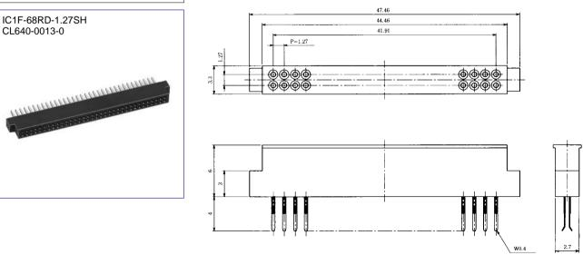
• Recommended board thickness : 0.4 to 0.5mm
