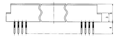
Recommended board thickness : 0.4 to 0.5mm
