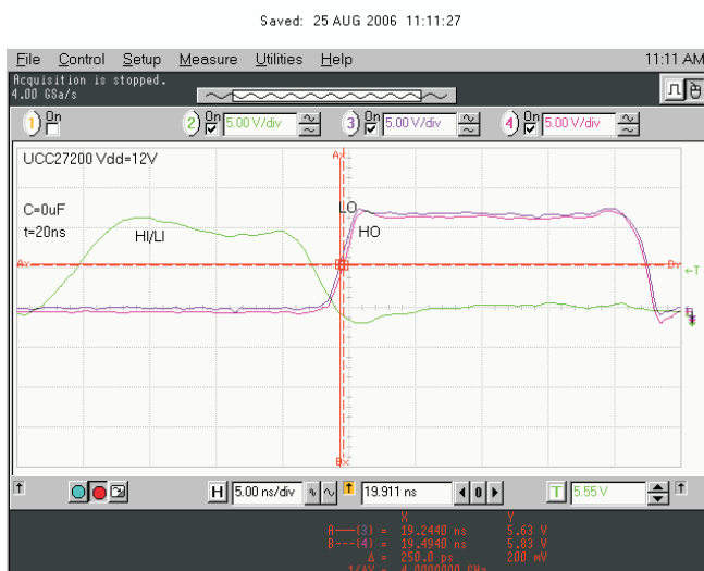
Figure 33. 20-ns Input Pulse Delay Matching
