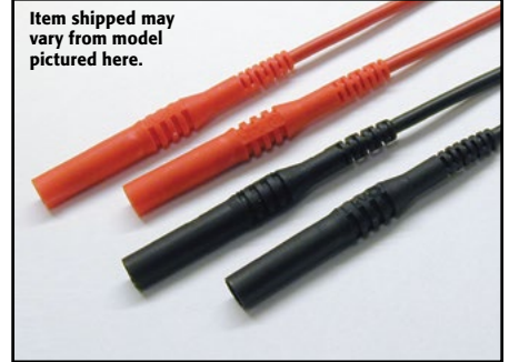
Model 8607 1kV Source Banana Cable Set: The 8607 cable set is made up of one red and one black high voltage test lead with fixed safety banana plug ends. The leads are 1 meter (3.3 ft) long and have a voltage rating of 1500V DC.
