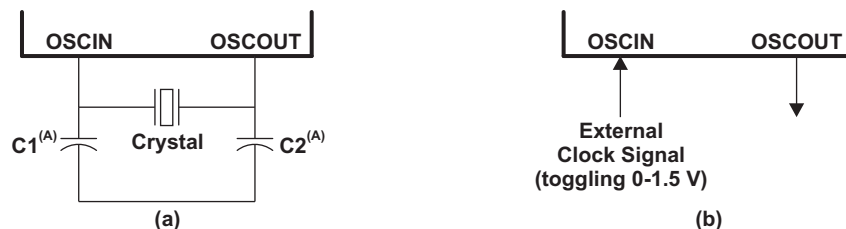
Figure 5-5. Recommended Crystal/Clock Connection
