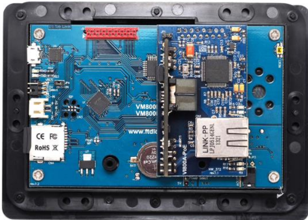
Figure 5-1 – VI800A-PoE module connected to VM800P Plus module
