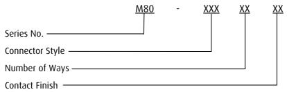
For details of styles, as well as Mix-Tek and M83 markings and styles see the latest catalogue, or individual drawings.
