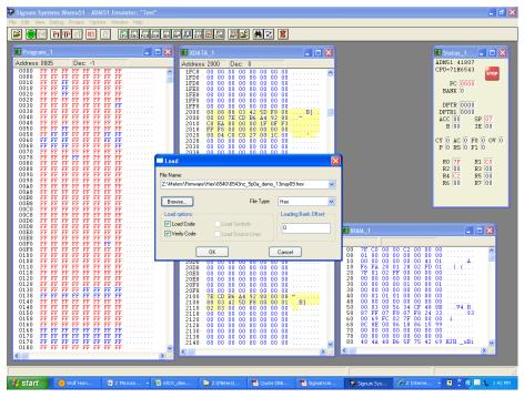
Figure 1-6: Emulator Window Showing Erased Flash Memory and File Load Menu
