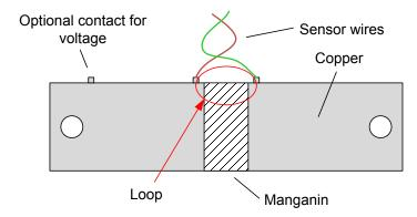
Figure 2-14: Loop Formed by Shunt and Sensor Wire
