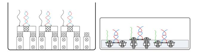
Figure 2-12: Typical Sensor Arrangement (left), Alternative Arrangement (right)
