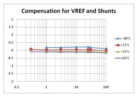
Figure 2-7: Wh Registration Error with Combined Compensation
