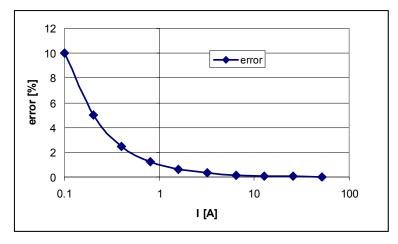
Figure 2-5: Non-Linearity Caused by Quantification Noise
