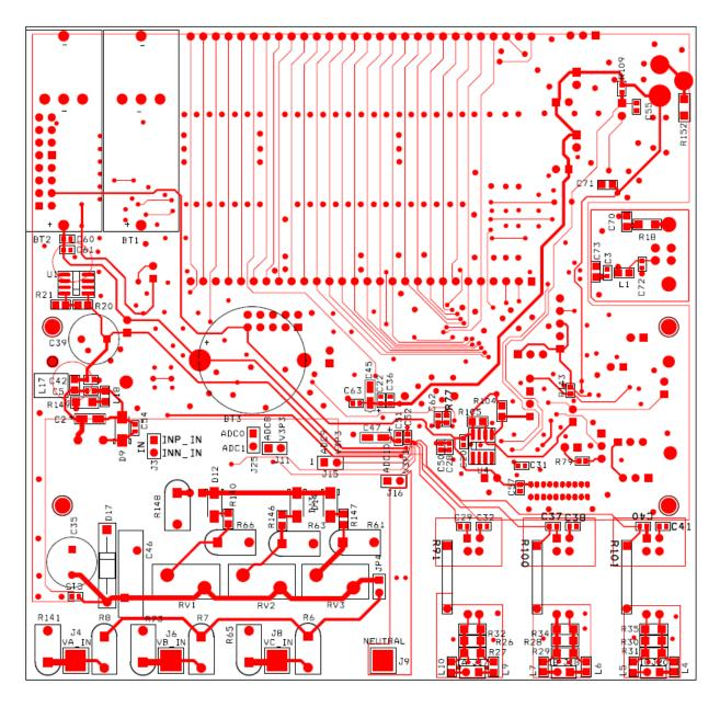
Figure 4-16: Teridian 71M6543 REV 5.0 Demo Board: Bottom View
