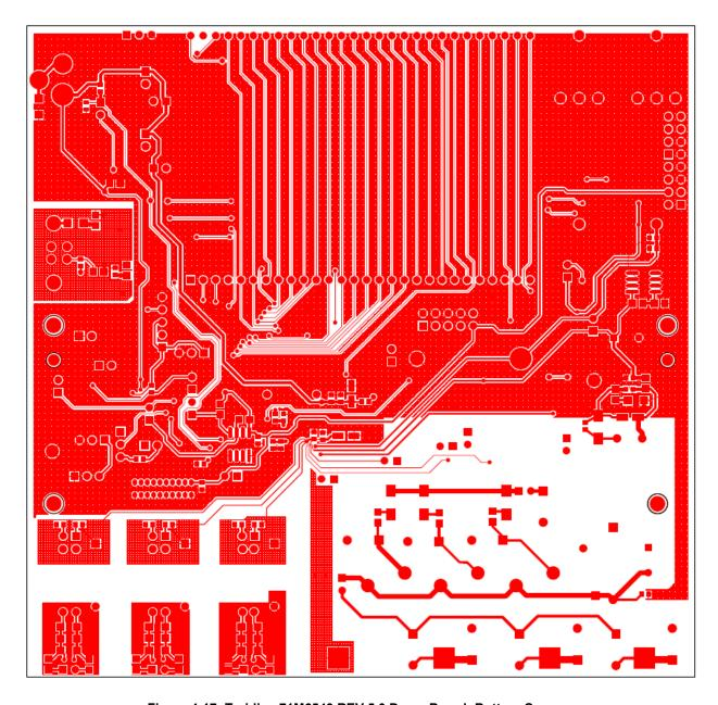
Figure 4-17: Teridian 71M6543 REV 5.0 Demo Board: Bottom Copper
