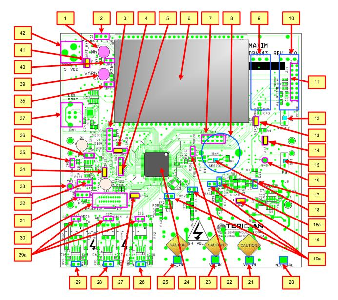
Figure 3-1: 71M6543 REV 4.0 Demo Board - Board Description
