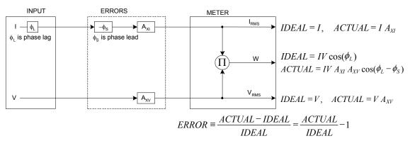
Figure 2-1: Watt Meter with Gain and Phase Errors.
