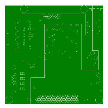
Figure 4-23: Debug Board: Middle Layer 2 (Supply Plane)
