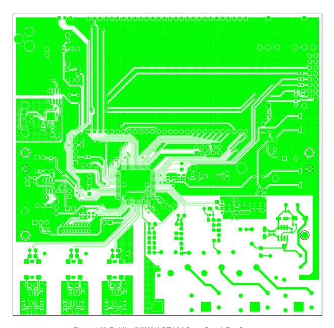
Figure 4-15: Teridian 71M6543 REV 5.0 Demo Board: Top Copper
