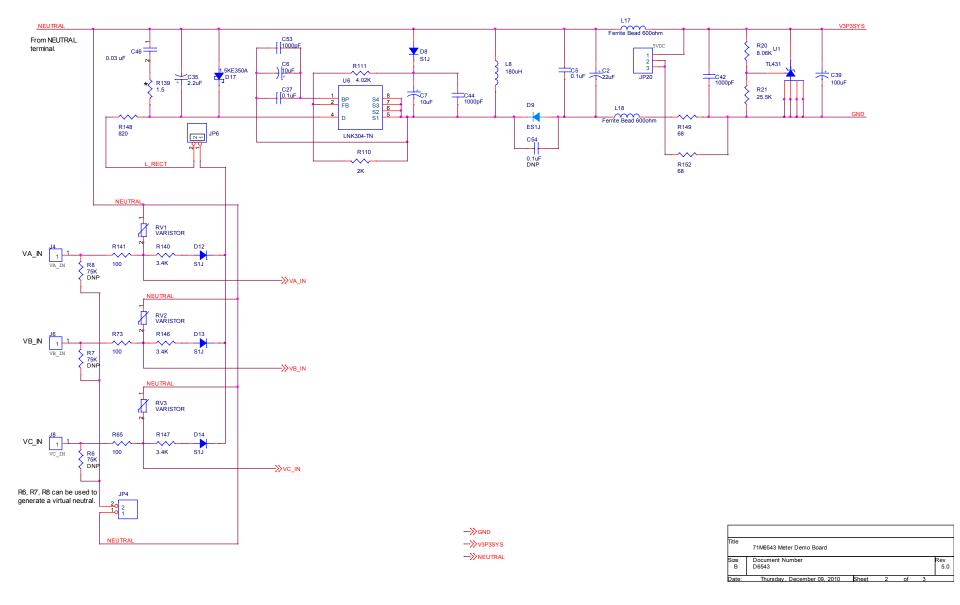
Figure 4-6: Teridian 71M6543 REV 5.0 Demo Board: Electrical Schematic 2/4
