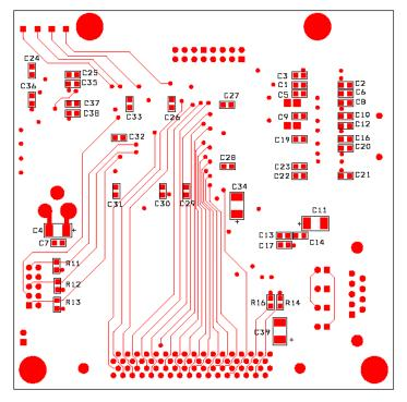
Figure 4-20: Debug Board: Bottom View
