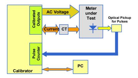
Figure 2-8: Meter with Calibration System
