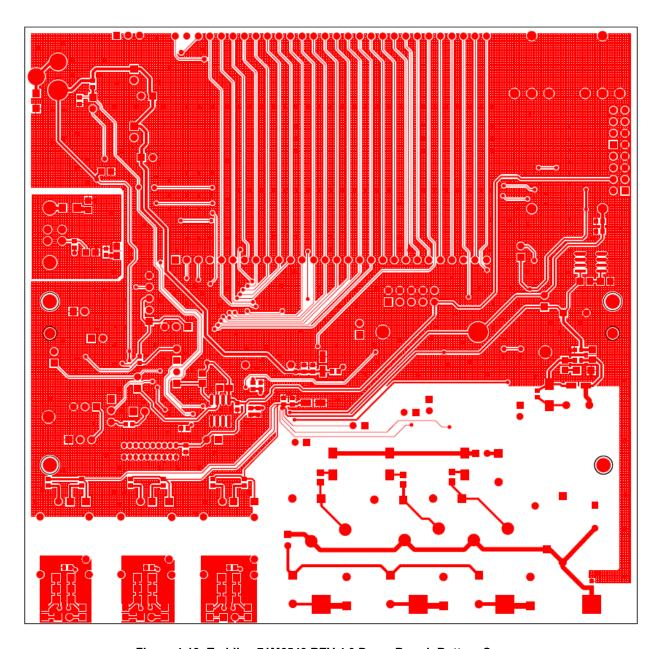
Figure 4-13: Teridian 71M6543 REV 4.0 Demo Board: Bottom Copper
