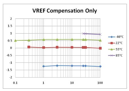
Figure 2-6: Wh Registration Error with VREF Compensation
