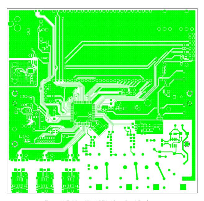
Figure 4-11: Teridian 71M6543 REV 4.0 Demo Board: Top Copper
