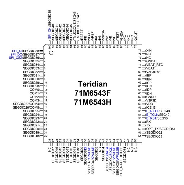
Figure 4-25: 71M6543, LQFP100: Pin-out (top view)
