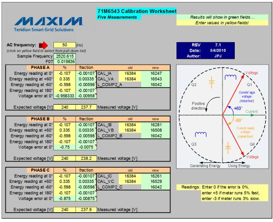
Figure 2-4: Calibration Spreadsheet for Five Measurements
