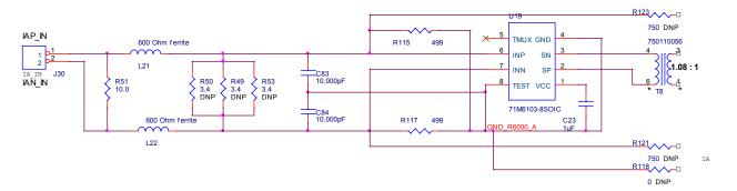
Figure 4-9: Input Circuit with Ferrites
