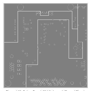
Figure 4-22: Debug Board: Middle Layer 1 (Ground Plane)
