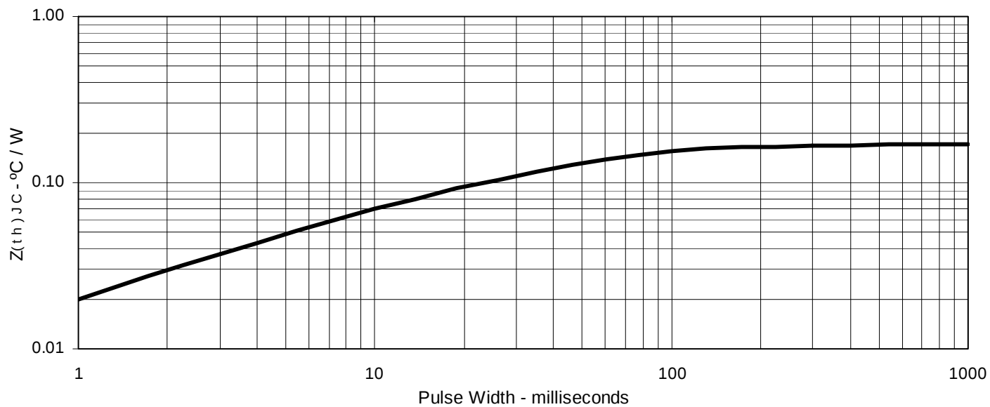
Fig. 13. Maximum Transient Thermal Impedance
