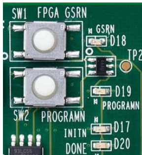
Figure 3. LatticeECP3 Status LEDs and Push-button Controls
