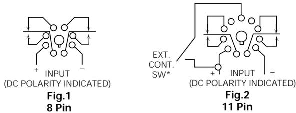
\* If control switch is closed when power is applied, relay will immediately energize. A 50 millisecond minimum switch closure is required. IMPORTANT: a dry circuit switch is recommended. A "dry circuit" switch is one rated to reliably switch currents of less than 50mA. Use of a switch rated for other than dry circuit may result in failure of the time delay relay to function properly.
