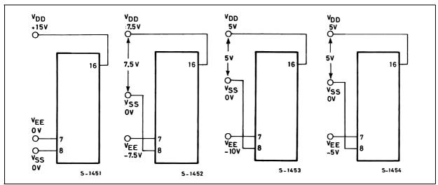
The ADDRESS (digtal-control inputs) and INHIBIT logic levels are : "0"= $V_{SS}$  and "1"= $V_{DD}$ . The analog signal (through the TG) may swing from  $V_{EE}$  to  $V_{DD}$
