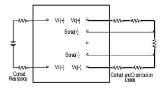
Figure 17: Effective circuit configuration for remote sense operation
