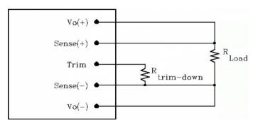
Figure 18: Circuit configuration for trim-down (decrease output voltage)
