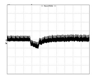
**Figure 8:** Output voltage response to step-change in load current (75%-50% of lo, max; di/dt = 0.1A/µs). Load cap: 10µF, tantalum capacitor and 1µF ceramic capacitor. Trace: Vout (20mV/div, 100us/div), Scope measurement should be made using a BNC cable (length shorter than 20 inches). Position the load between 51 mm to 76 mm (2 inches to 3 inches) from the module..
