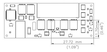
**Figure 21:** Case temperature measurement location. Pin locations are for reference only. \* The allowed maximum hot spot temperature is defined at 130  $^{\circ}$ C
