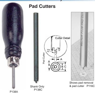
Vector Pad Cutters provide an effective method for creating isolated solder pads around holes in copper clad boards. Pilot pin enters hole and rotates, creating a clearance area around the solder pad. Available for boards with.062" or .042" diameter holes. Also available without handles for use with manual or power drills.
