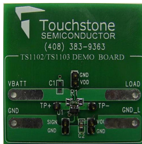
Figure 2. TS1103 Demo Board
