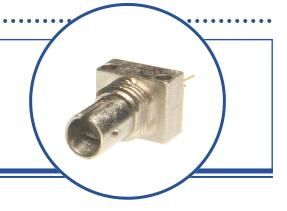
The OPF397 family fiber optic transmitters are high performance devices packaged for data communication links. This transmitter is an 850nm GaAlAs LED and is specifically designed to efficiently launch optical power into fibers ranging in size from 50/125µm up to 200/300µm diameter fiber. Multiple power ranges with upper and lower limits are offered which allows the designer to select a device best suited for the application.
