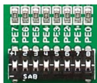
Figure 6-2: Tri-state DIP switch on PORTE
