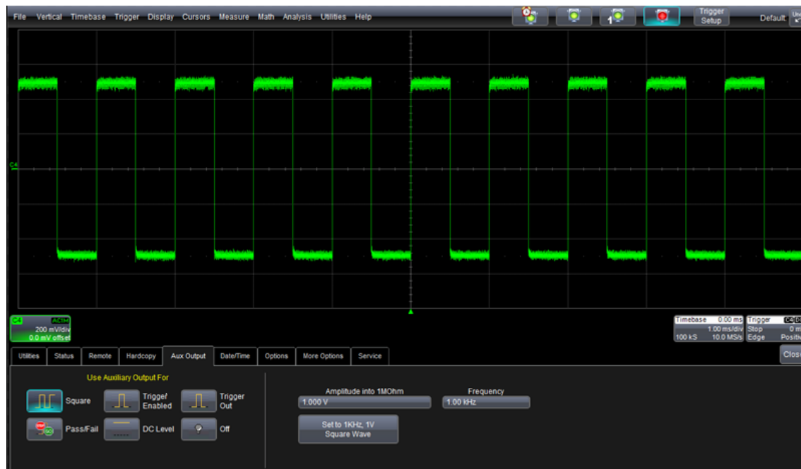
Figure 5-4. Square wave output signal
