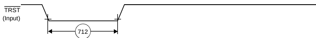
Figure 29. TRST Timing Diagram
