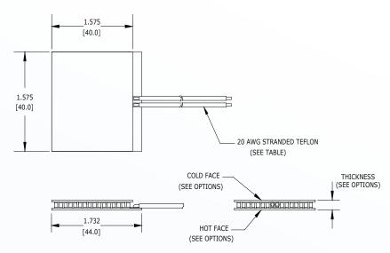
Ceramic Material 96% Alumina Ceramics Solder Construction: 138°C BiSn
