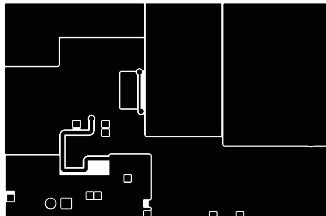
Figure 41. TPS40200EVM-001 Bottom Copper (X-Ray View from Top)
