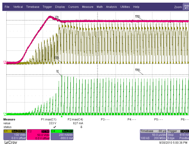
Figure 38 – 115 VAC / 60 Hz, 90° Dimming Phase Angle. 6 LED in Series (18.2 V / 350 mA) Ch1(Yellow): V_{DS} , 100 V / div. Ch2(Red): V_{IN} , 50 V / div. Ch4(Green): I_{DS} , 200 mA / div., 50 \mu s / div.
