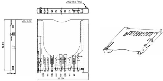
Mini Connector: Bottom Mount, Push/Push Insertion/Removal
