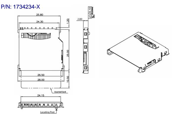
Full Size Connector: Top Mount, Push/Push Insertion/Removal
