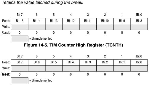
If you read TCNTH during a break interrupt, be sure to unlatch TCNTL by reading TCNTL before exiting the break interrupt. Otherwise, TCNTL
