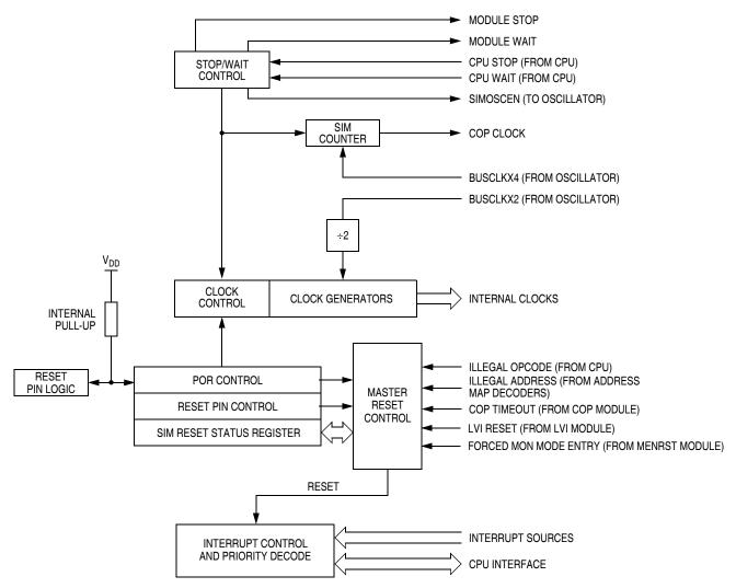
Figure 13-1. SIM Block Diagram
