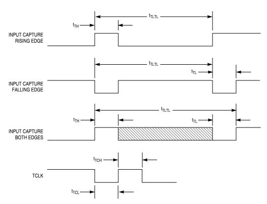
Figure 16-11. Timer Input Timing
