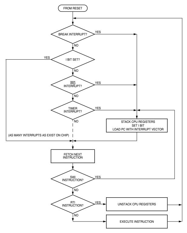
Figure 13-7. Interrupt Processing
