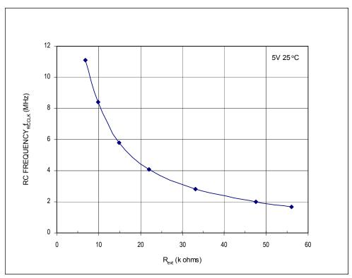
Figure 16-7. RC versus Frequency (5 Volts @ 25°C)
