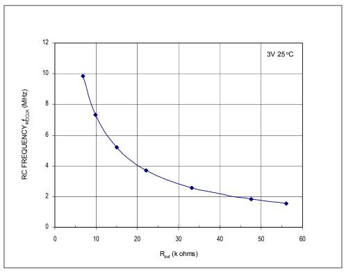
Figure 16-8. RC versus Frequency (3 Volts @ 25°C)
