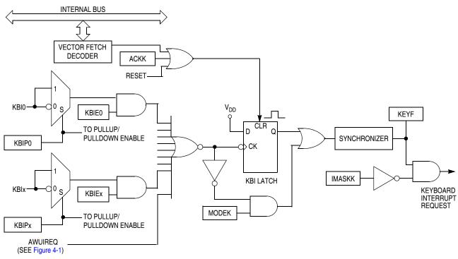
Figure 9-2. Keyboard Interrupt Block Diagram
