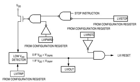
Figure 10-1. LVI Module Block Diagram
