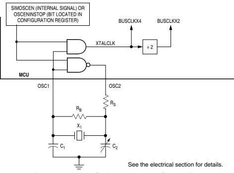
Figure 11-2. XTAL Oscillator External Connections
