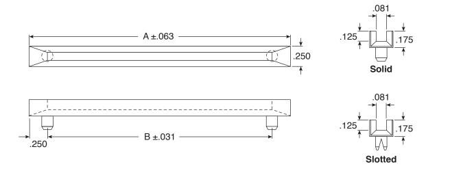
Printed circuit board support guides are an economical and fast solution to mount P.C. Boards. Card insertion is simple and fast. The smooth positive channel guides the P.C. Board and firmly supports and protects the board. Guides are molded of tough, electrically insulating nylon 6/6 and are designed to snap into pre-punched holes in the chassis.
