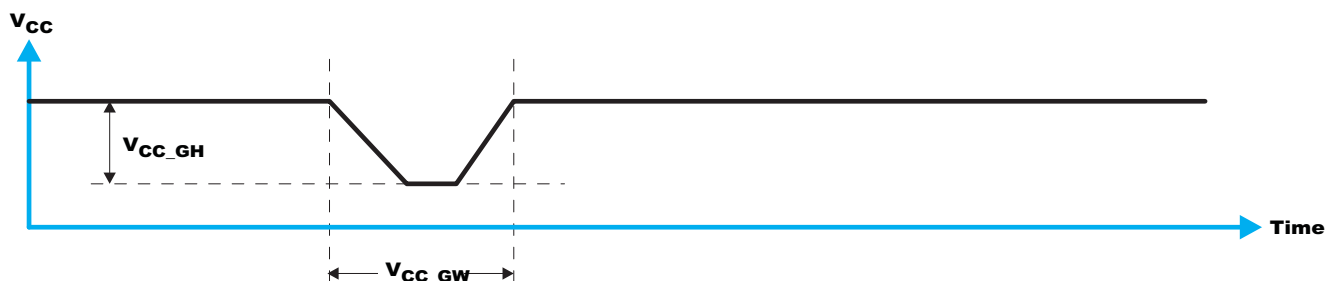
Figure 30. Glitch Width and Glitch Height
