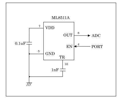
\* Load resistance of OUT port is recommended more than 100 k $\Omega.$
