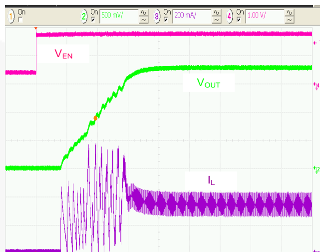
Figure 18. Soft-Start, R_{LOAD} = 6\Omega , 20μs/div.
