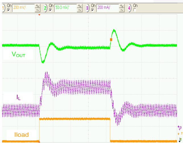
Figure 15. Load Transient 200 to 500mA, 3.6VIN, 5µs/div.
