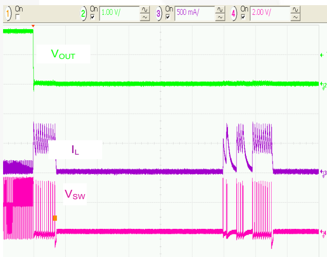
Figure 16. Metallic Short Applied at VOUT, 50µs/div.
