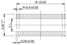
Recommended solder paste thickness: 120  $\mu$ m
