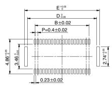
Recommended solder paste thickness: 120  $\mu$ m
