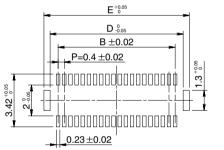
Recommended solder paste thickness: 120  $\mu$ m
