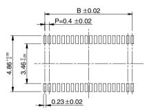
Recommended solder paste thickness: 120  $\mu$ m
