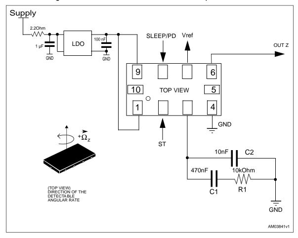
Power supply decoupling capacitors should be placed in combination with an LDO regulator (common design practice).
