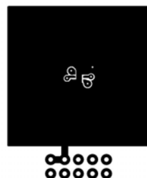
c. 69\text{ }^{\circ}\text{C/W} when mounted on a 1 in 2 pad of 2 oz copper
