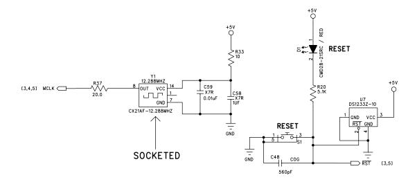
Figure 7. Reset Circuit
