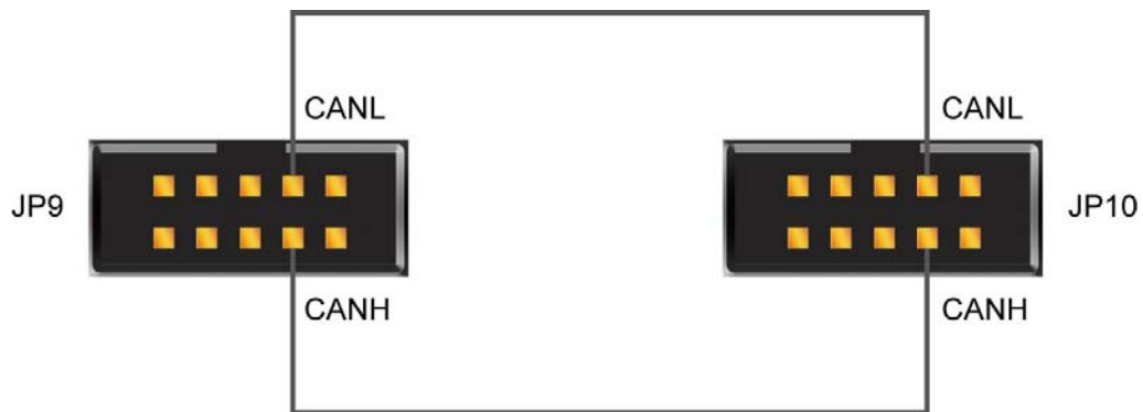
Figure 5-7 Wiring for CAN loopback test
