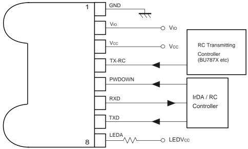
(2-a) RC transmitting mode at IrDA receiver active condition.
