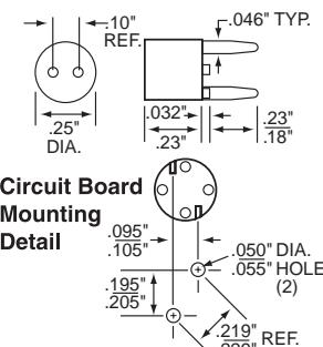
Fuseholder will accept Littelfuse MICRO™ fuses and PICO® II fuses (rated to 5 amperes) with .025" diameter leads.
