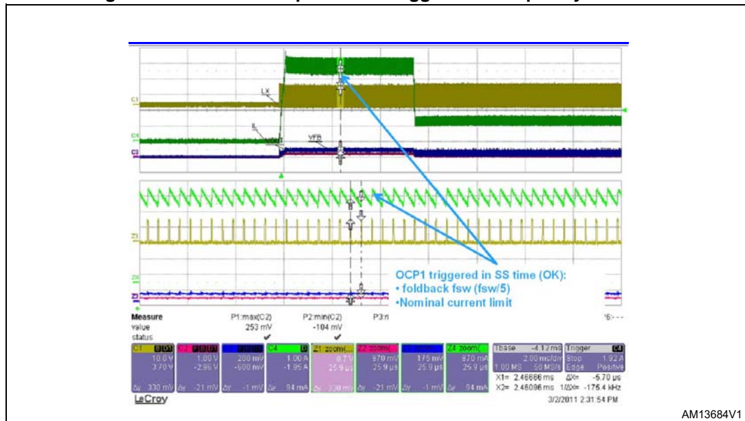
Figure 23. Over current protection triggers the frequency foldback
